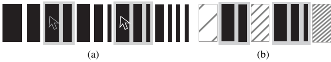
Fig. 4. Diagonal stripe glyphs. (a) Selecting the root nodes of two subtrees of interest; (b) Replacing each contiguous uninteresting region with diagonal stripe glyphs. The density of the diagonal stripe texture in each glyph encodes the number of elided nodes.
