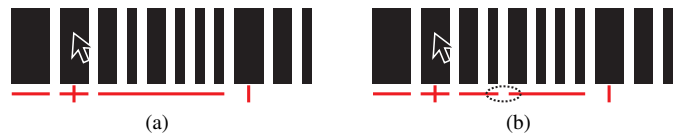
Fig. 3. “Structural cues” highlight certain nodes in response to the cursor hovering over a node, to make topological relationships more apparent. Horizontal underlining appears under ancestors to the left of the cursor, and also under descendants to the right of the cursor. Vertical tick marks appear under siblings at the same level as the node under the cursor. Both marks appear under the node under the cursor, resulting in a cross-shaped glyph. Above we see two variants of these structural cues, with an ellipse with dotted border indicating their differences: (a) Descendants are shown with a single horizontal stroke; (b) Each subtree is shown with a separate stroke.
